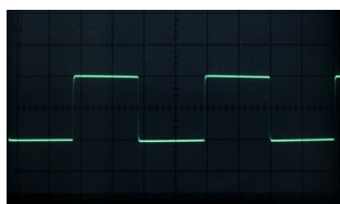
Fig.2 Square Wave 1KHz*
